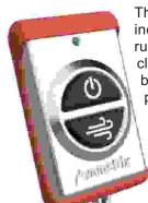
The AvyScanner includes a small, rugged fob that clips to your backpack to provide air temperature and estimated wind speed.
